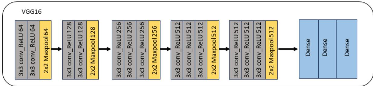
Figure 3. Architecture of VGG16
